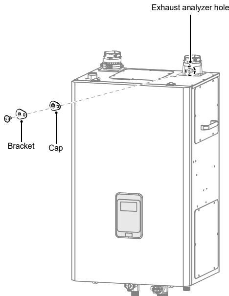
**13** Insert analyzer into the exhaust analyzer hole and measure the gas/air ratio (using combustion analyzer is recommended).
