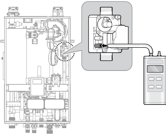
**6** Re-open the manual gas shut-off valve and check for leaks.
