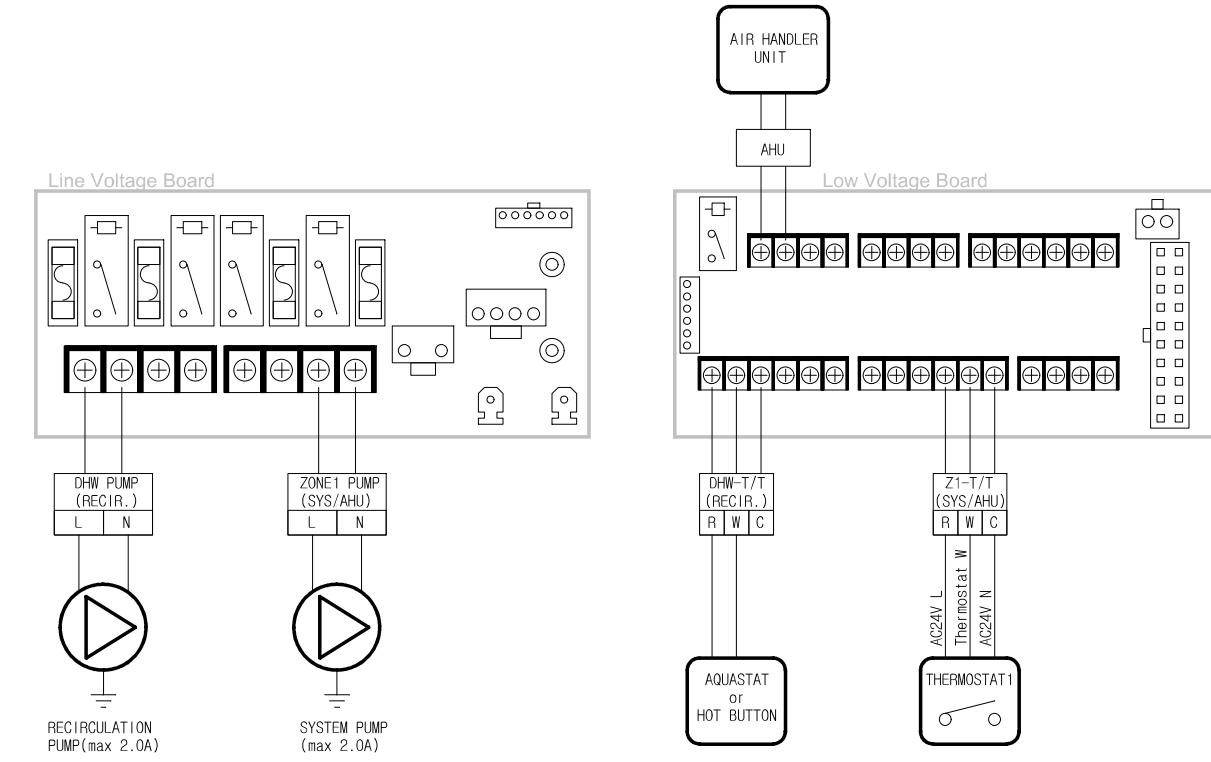
◎ Connect the pump ground to the front chassis.
