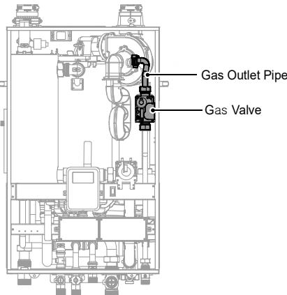
4 Loosen the nut connecting the gas outlet pipe and the gas valve. Carefully separate the clip.
