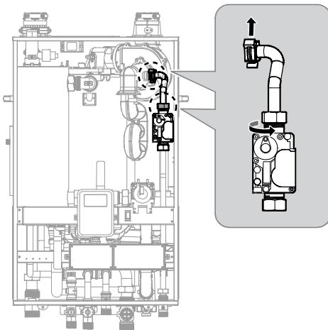
5 Once the gas orifice is exposed, remove the gas orifice from gas valve.
