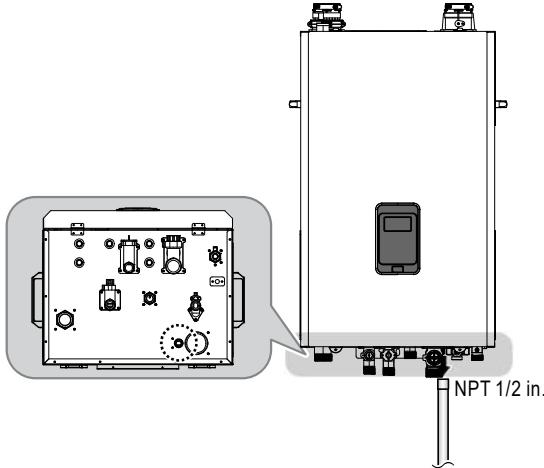
2 Place the free end of the drain line into an appropriate drain.
