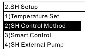
2 Set either Supply Based or Return Based as SH Control Method.
