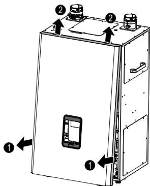
**10** Replace the front cover and tighten the 2 Phillips screws to secure it to the case.
