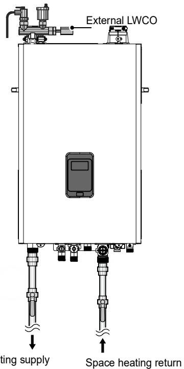
LWCO installed outside should be installed at least 6 inches (150mm) or more away from the end of the heat exchanger.
