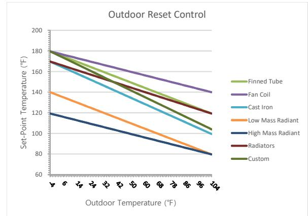
Space Heating Temperature Setting for the Outdoor Reset Control
