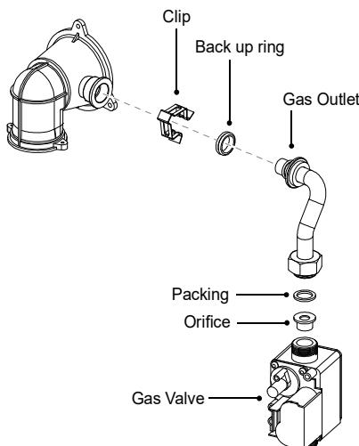
6 Replace the old orifice piece and the packing with new part for use with Propane. Ensure that the orifice is properly seated inside the gas valve
