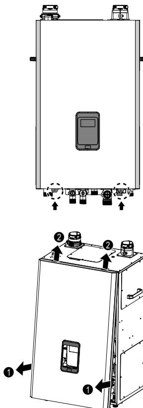
3 Once the front cover is removed, place it in a safe location to prevent accidental damage. With the internal components exposed, locate the gas connector and the gas valve.
