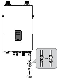
**2** Run space heating. The boiler should turn on and the gas in the gas supply line will be purged.
