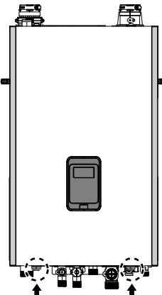
**8** When the boiler reaches its maximum firing rate, check the inlet gas pressure reading on the manometer. The gas pressure must fall within the ranges specified in "Specifications" on page 7.
