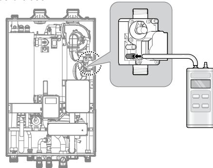
**6** Re-open the manual gas shut-off valve and check for leaks.
